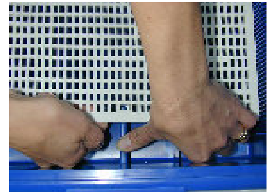
Picture 12 - Base grille removal
